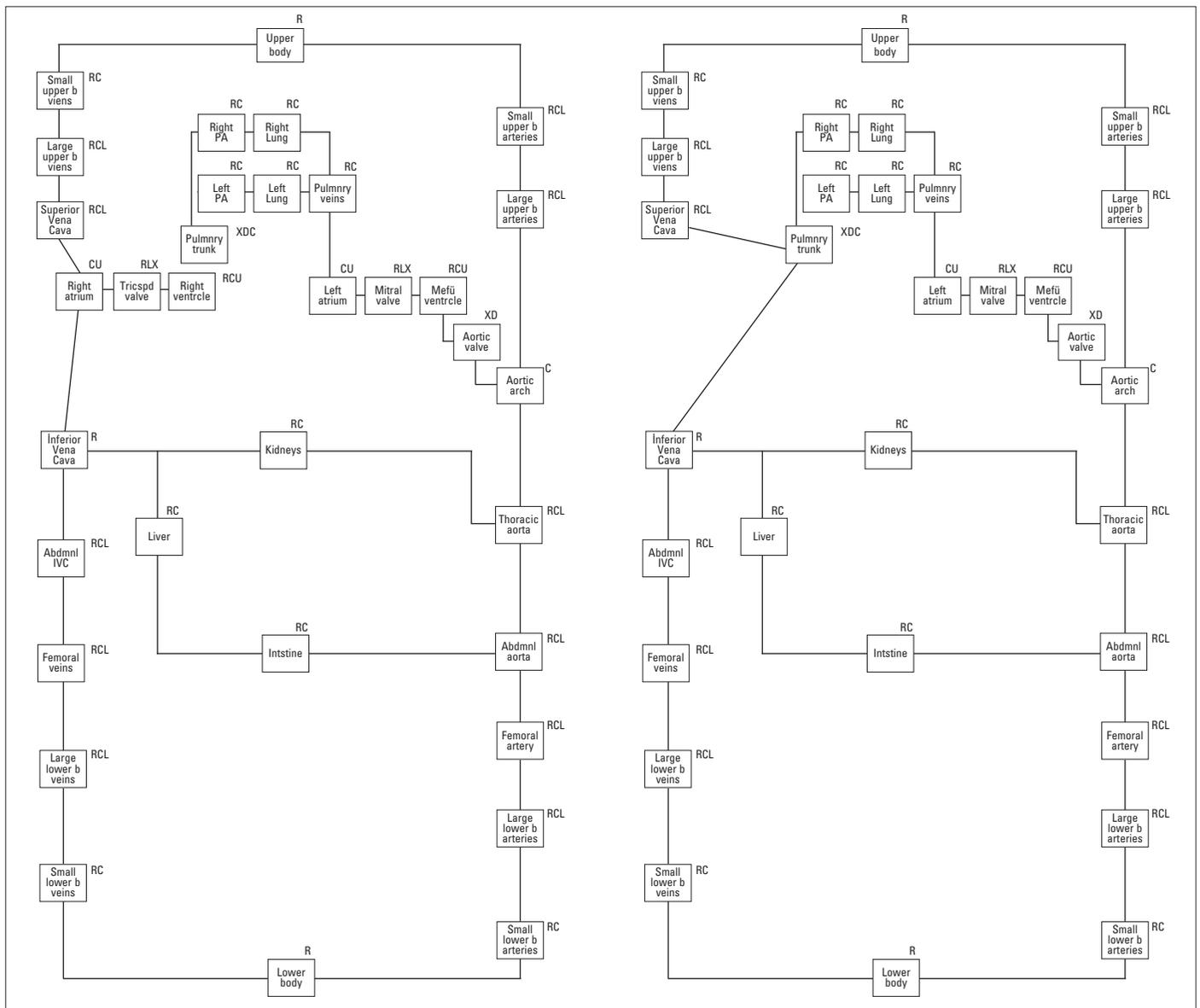
**Figure 1.** Schemes of lumped parameter models for the healthy paediatric circulation (left) and the total cavo-pulmonary connection arrangement (right). Letters near each block represent parameters built in the block. R: hydraulic resistance; C: blood vessel compliance; L: blood inductance; D: localised energy loss; X: valve function; U: pressure generator.
