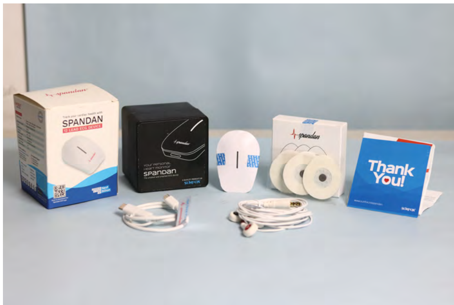
Figure 1. Spandan portable electrocardiogram, developed by Sunfox Technologies Pvt. Ltd., is a smartphone-based portable ECG device capable of taking lead II and also 12 lead ECGs by using derived ECG methods to evaluate cardiac arrhythmias.
