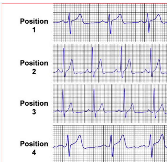
Figure 3. ECG recordings of novel device from different electrode positions
