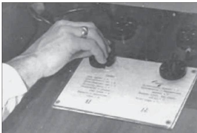
Figure 4. The switch of the channels, submitting various sound signs and the sound standards. Under the switch is the list of channels and sounds phenomena. If the TM fixed an error, a student has compare of his personal sound task with each sound standard at any moment, and after correction has continued of his DT. So actually sounds signs programmed training to its correct recognition have been combined
